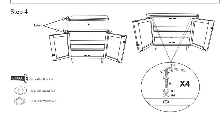
Position Top Frame (A) onto assembly. Ensure that the holes of all components align and that the labels match accordingly (C1 with C1). Secure the connections using Allen Bolts (H-1), Lock Washers (H-3) and Flat Washers (H-2), stacking the hardware in the order as shown. Engage all hardware, Then fully tighten all hardware from this and previous steps using provided Allen Key (T-1). Do not over tighten.
