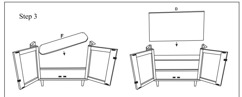
Position the Inner Shelf (F) from the top as illustrated, ensuring that the corner cutouts are toward the back. Once in position, slide the Back Panel (D) into the grooves on the backside of the door panels.
