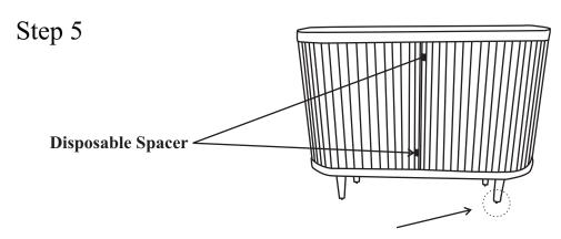
NOTE: Levelers can be used for adjustment if needed.
